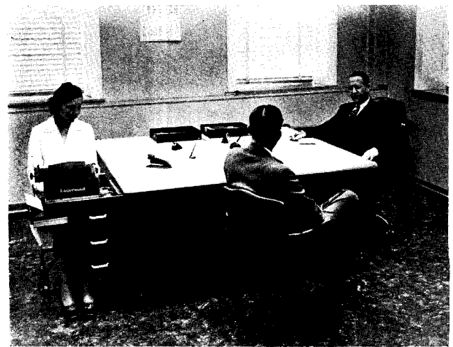
Figure 6: This desktop, with a reflection-factor of about 30 per cent, provides better seeing conditions than dark ones. The author recommends the idea generally for business equipment
