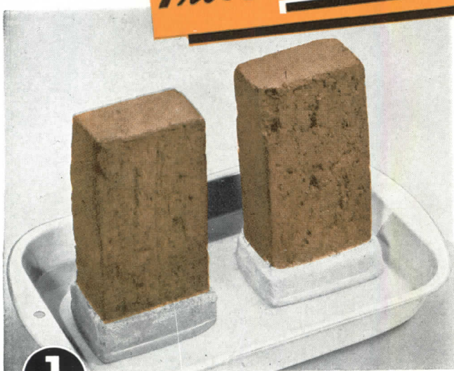
"Cap" one brick with Brixment mortar (left), and one brick with mortar made with 50-50 cement and lime. After mortars have hardened, place both brick in a pan of shallow water. (Photo 1.)
