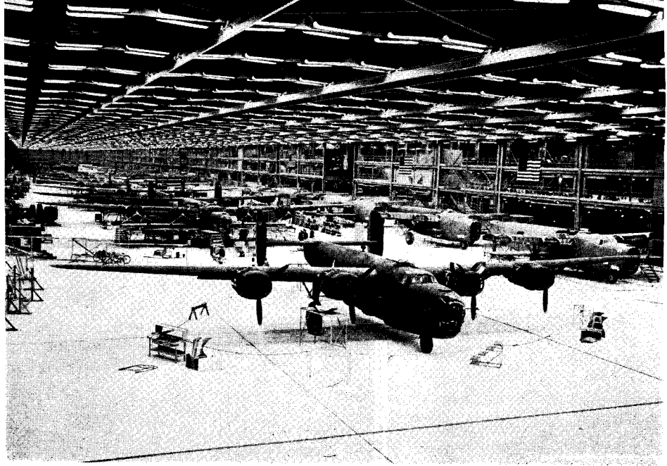
Figure 10: The photograph conveys some small idea of the contribution toward good seeing conditions of a light floor (this floor of "white" cement has a reflection-factor of about 40 per cent). Design and construction by The Austin Co.
