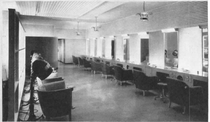
A Beauty Shop in Saks Fifth Avenue, Chicago, provides soft flattering light over the dressing tables, through Satinol Flutex panels, lighted from behind. Architect, James F. Eppenstein.
