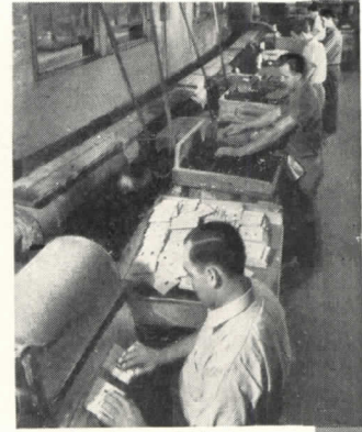
Sanding Operation, where Bakelite pieces from the presses are cleaned of burrs and fins by manipulation on sand belts.
