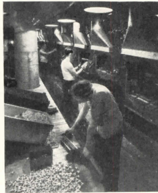
Air-compressed Semi-automatic Molding Presses, utilized for the shorter runs and particularly where extreme accuracy is required in the smaller parts.
