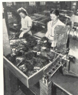
Automatic Cleaning Fixture for finishing wall plates. This machine removes used flash, left in holes during the pressing operation.
