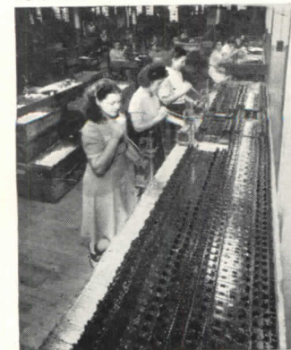
Automatic Cleaning Fixture for finishing wall plates. This machine removes used flash, left in holes during the pressing operation.
