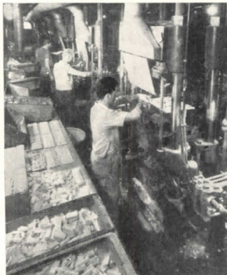
Hydraulic Presses making wall plates. These machines apply a pressure of 160 tons per sq. inch, and produce 15 plates on one closing of the molds.
