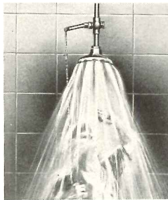
S-2075—SPEAKMAN Emergency Shower. Size, 1 inch. Cast brass, self-cleaning adjustable shower head. Supply from ceiling with flange and slow self-closing valve, heavy chain to floor and floor flange.
