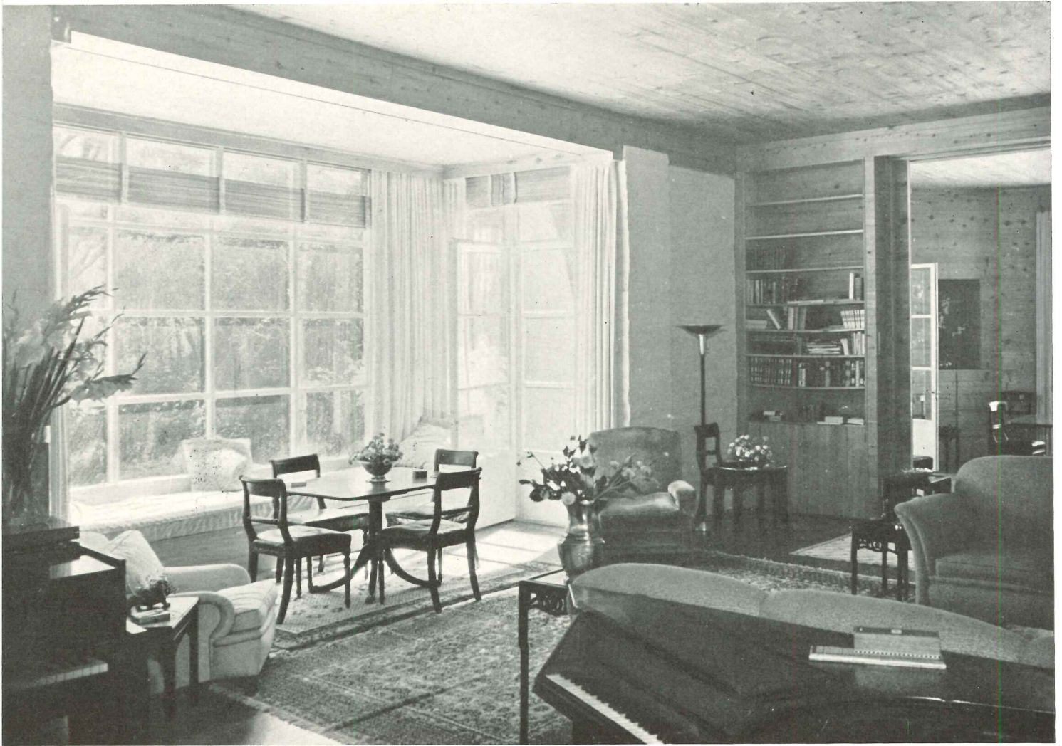
Above, interior of living-room; below, dining-room. All same walls are finished with knotty red cedar board-and-batten. Wood studs and plates are secured to adobe walls with bent lengths of barbed wire embedded in mortar joints and nailed to framing.
