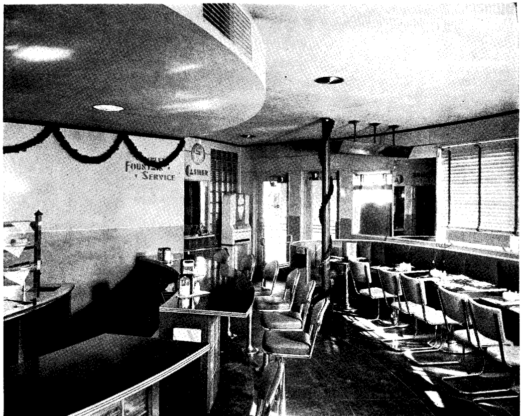
Dining room looking toward cashier's booth and entrance and exit doorways. The dropped ceiling in the center of the room acts as a plenum chamber for the air-conditioning system. Furnishings are of chrome steel with antique white and coral Fabricoid upholstery.
